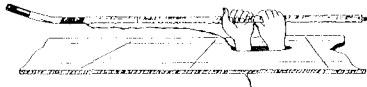
Artist conception of how rods are joined together above ceiling to PUSH wire from one point to the next point.
